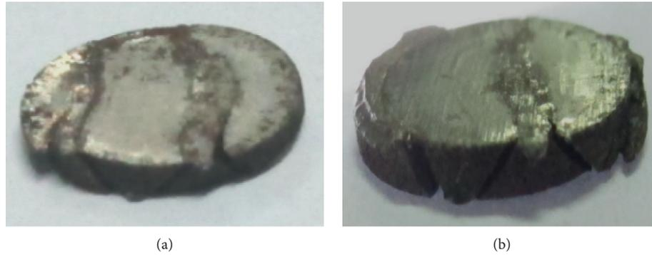
FIGURE 14: Recycled specimens for dynamic compression experiments at varying temperature. (a) QP980 steel RSW; (b) TRIP800 steel RSW.
