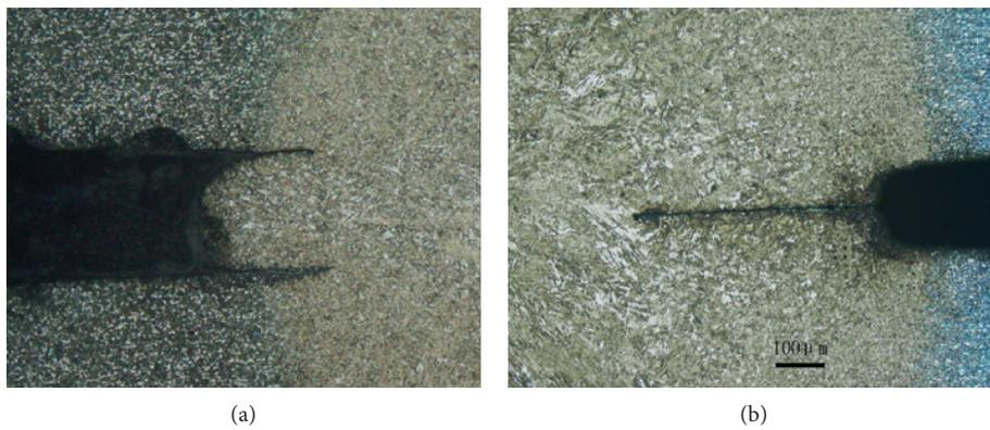
FIGURE 9: Weld line. (a) QP980 steel RSW; (b) TRIP800 steel RSW.
