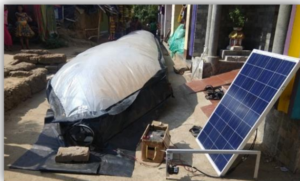
Fig. 2. Components of solar bubble dryer
