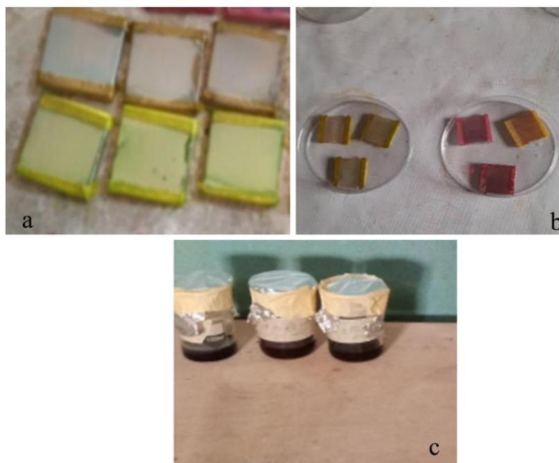
**Fig. 2. Pictures of (a), (b) Dye sensitized films, (c) Sintered substrates immersed in the dye sensitizers covered with aluminium foil.**
