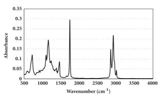
FIGURE 3: ATR-FTIR spectrum of Croton oil from Sipili, Kenya, before baseline subtraction and normalization to the C=O stretch at 1743 cm<sup>-1</sup> attributed to the ester carbonyl of the triglycerides.
