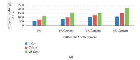
FIGURE 6: UCS of RM-FA reinforced with cement.
