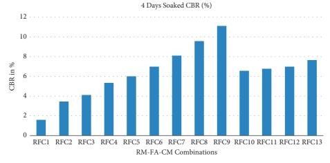
FIGURE 5: CBR values of RM-FA reinforced with cement.
