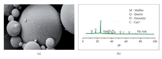
FIGURE 4: (a) SEM of fly ash and (b) XRD of fly ash.
