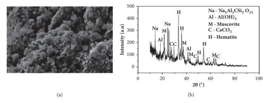
FIGURE 3: (a) SEM of red mud and (b) XRD of red mud.
